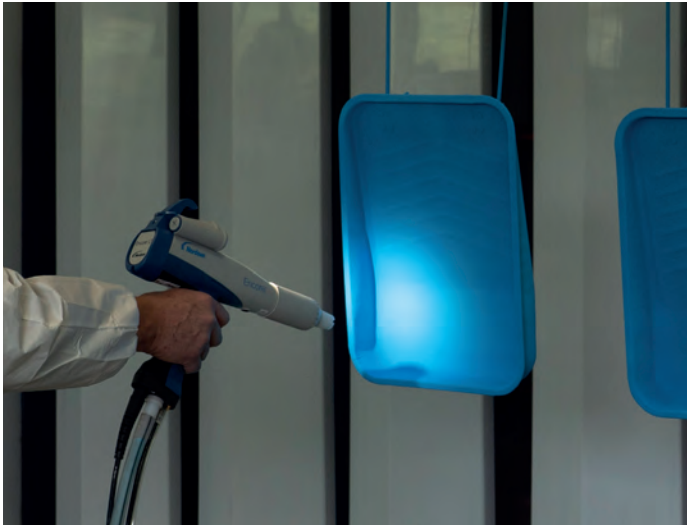
Encore nLighten LED kit – light on. Focused light beam for easy inspection during and after spraying.
