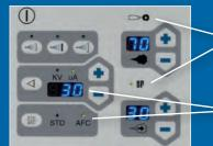
Green LEDs indicate Smart Flow mode, gun triggered on
