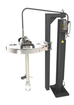
This elevator-agitator for 20-40 to 200 Liter drums features a double-effect jack for a fast lift of a stainless steel cover fitted for a quick material drum change. The cover is equipped with a motorized agitator fitted with blades for low viscosity materials and a full stainless steel rod. The elevator is coming on a large fixing plate which makes it very stable and easy to install in paint kitchens, existing installations or an essential component of new installations
