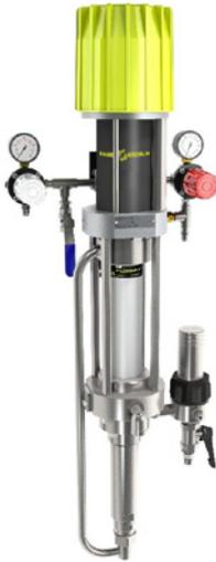
This 20F50 paint pump uses Flowmax® technology for total sealing, performance and extended lifetime for Airmix® applications.
